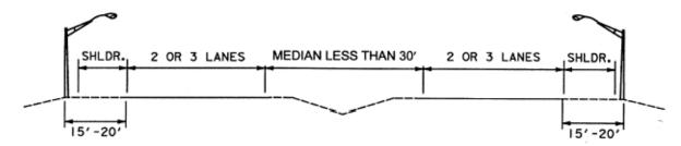
Figure 6-4. Typical house-side lighting for controlled access highway. In this example: Luminaires are 250W EQ LED - Mounting Height is 40 feet. - Spacing varies (see Section 6 of this chapter, Spacing of Light Poles).
