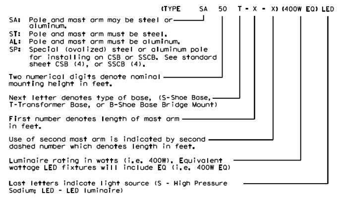
*Figure 5-1. Explanation of roadway illumination assembly codes.*
