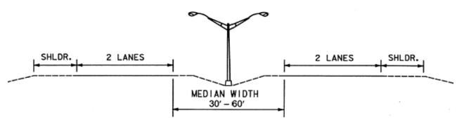
Figure 6-5. Median lighting with breakaway poles.
