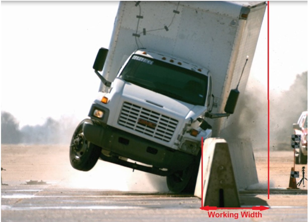
Figure A-2. Working Width
