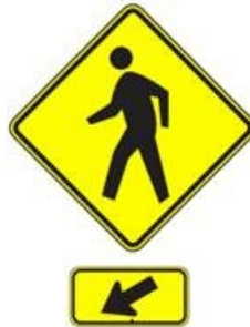
Figure D-3. Supplemental Crosswalk Signs W11-2 and W16-7PL Sign and Plaque ( TMUTCD )
