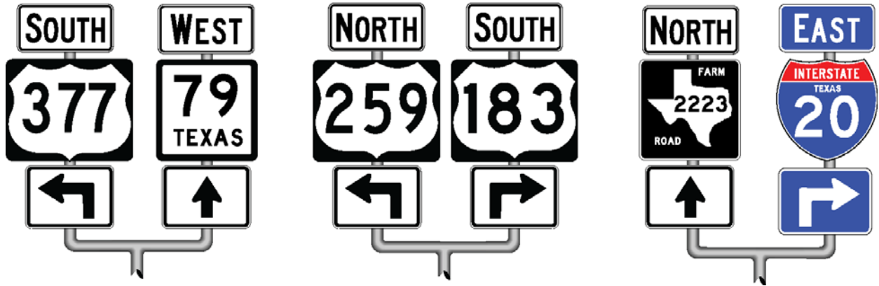
Figure 3-25. Advance Route Turn Assembly
