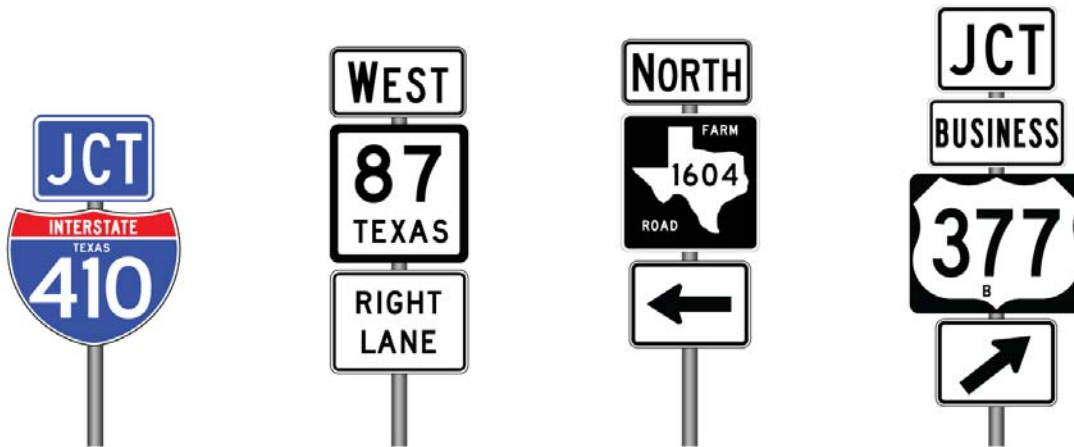
Figure 3-15. Examples of a Guide Sign Unit
