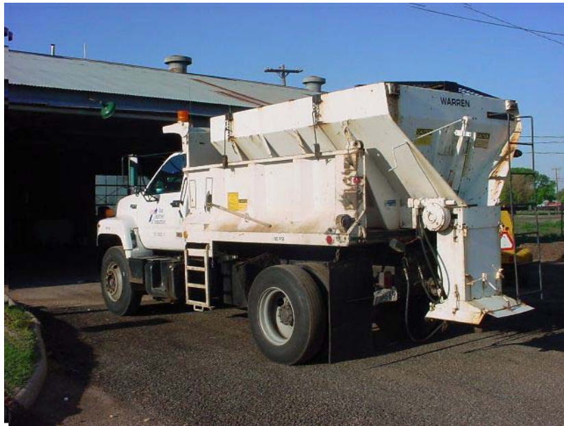
Figure 3-6. Tail gate spreaders are used to apply de-icing and anti-icing materials. They are a spinner type applicator and operate via a hydraulic system.
