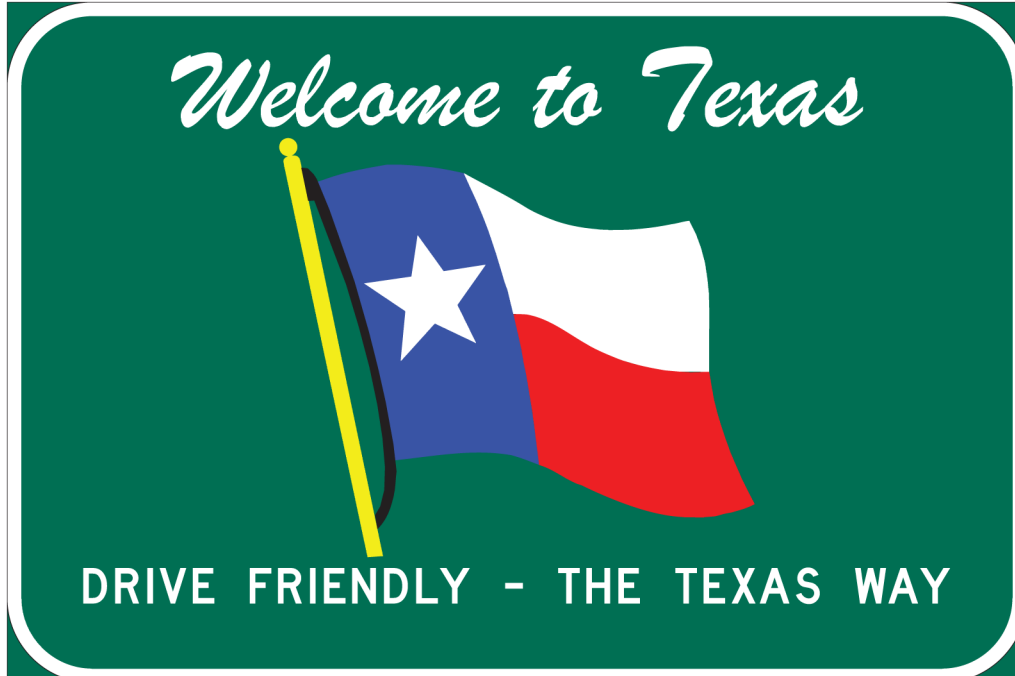
Figure 7-16. WELCOME TO TEXAS (I-2T) sign for interstate highways
