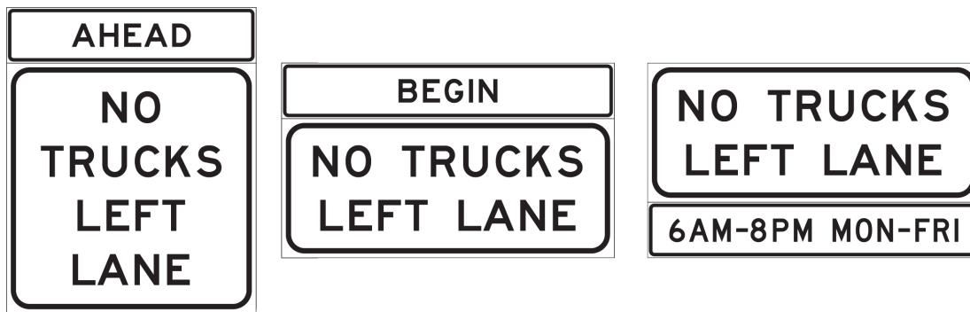
Figure 5-12. Typical sign examples of left lane truck restriction sign with plaques
