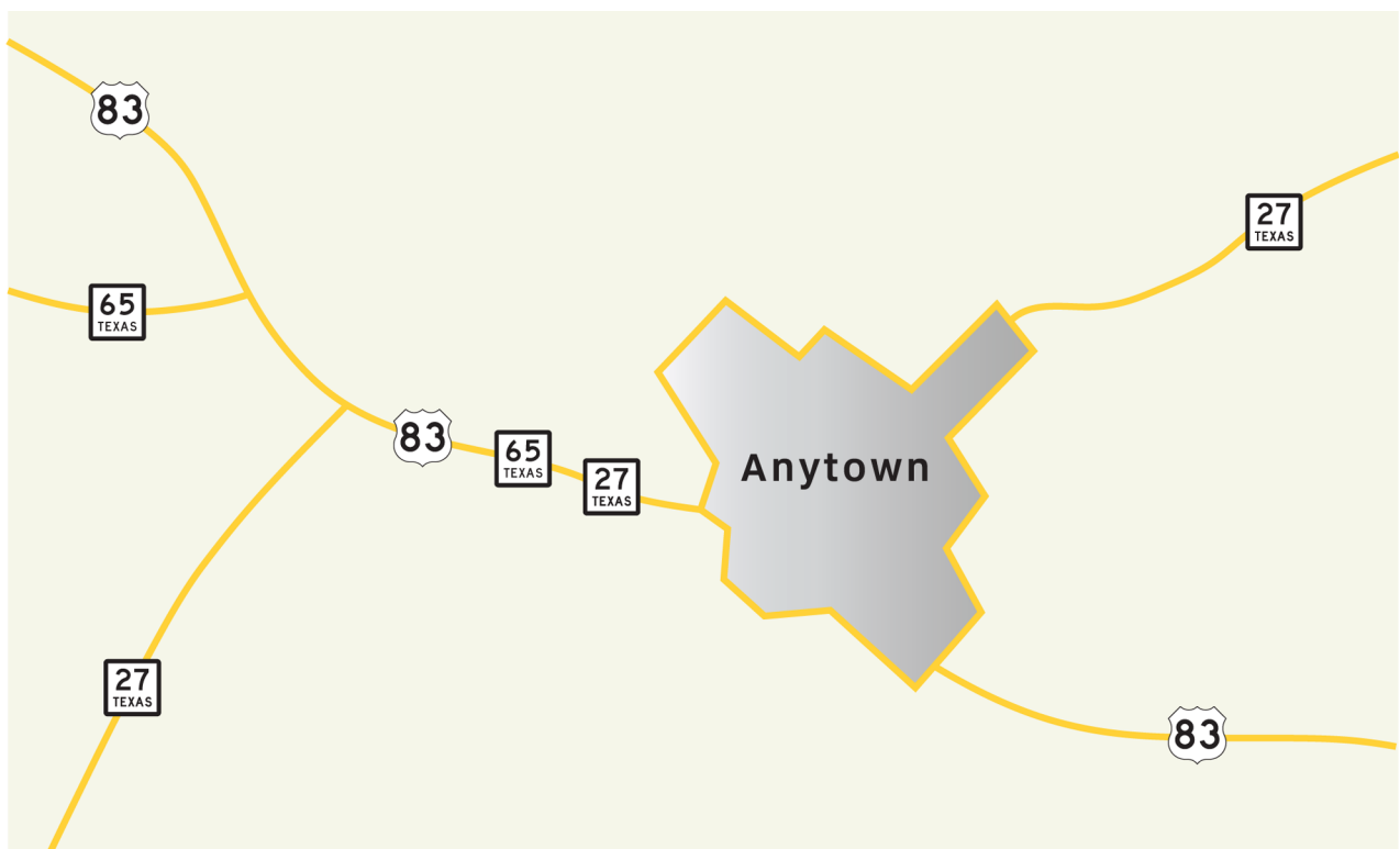
Figure 7-1. Example of unnecessary concurrent signing. Signing for SH 65 should terminate at junction with US 83.
