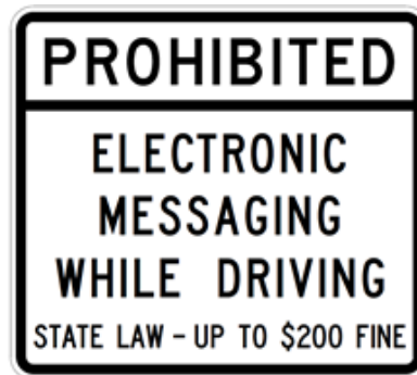
Figure 8-5. R19-6bT Electronic Messaging While Driving Prohibited Sign
