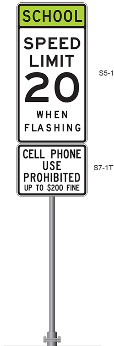
Figure 8-6. Example of Cell Phone Use Prohibited sign assembly.
