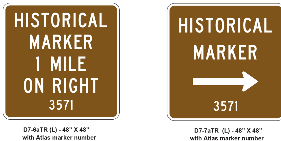
Figure 7-12. Advance and directional historical marker guide signs with Atlas marker numbers. Colors: legend - white (retroreflective); background - brown (retroreflective).
