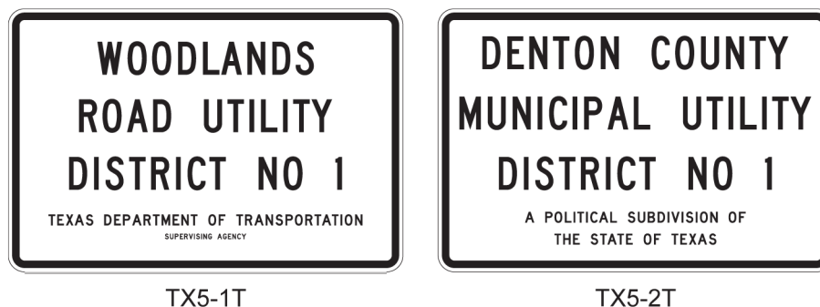
Figure 8-3. Typical utility district signs. Background is white reflective; border and legend are black. The three upper lines are for the district name. Variations in the number of letters per line will depend on the length of the district name.
