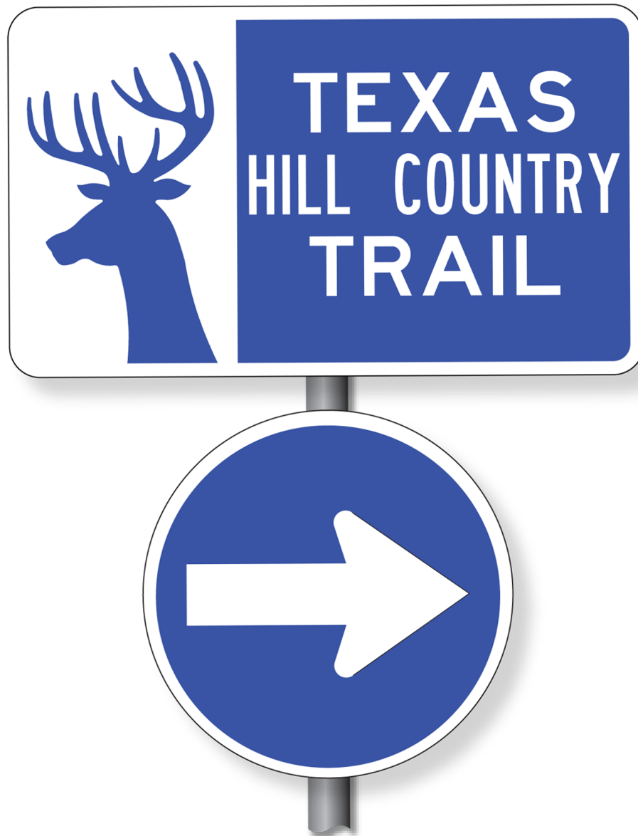
Figure 7-3. Example of Texas Heritage Trail Marker (Trail arrow may be reversed for left turn.)
