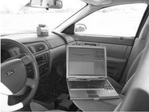
Figure 5-3. Equipment setup in test vehicle-laptop positioning.
