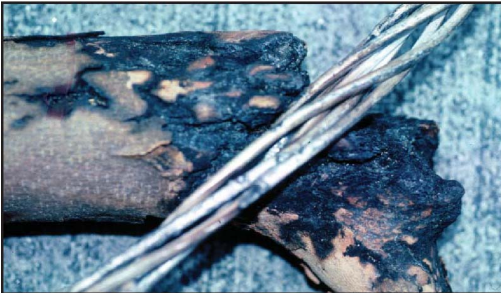
Figure 4-17. Tree limb in contact with high-voltage utility conductor line.
