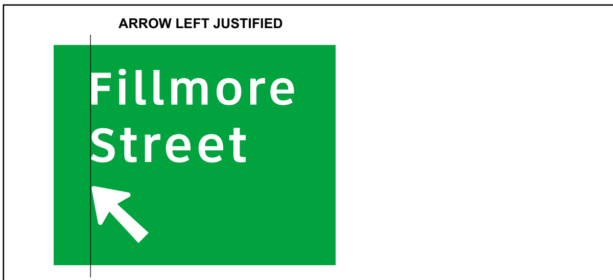
Figure 4-40. Arrow placement with roadway designation on the second line of copy.
