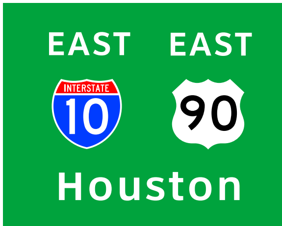
Figure 4-31. Placement of two Route signs with the same cardinal direction.
