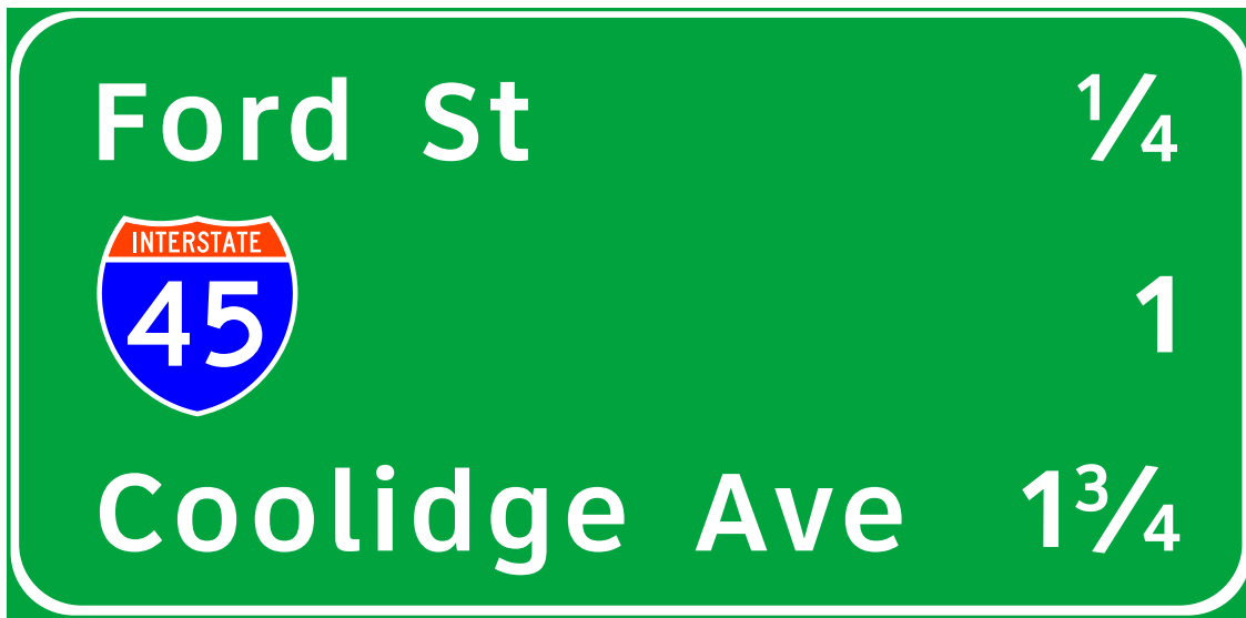
Figure 3-4. Interchange Sequence sign.
