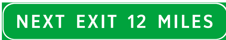
Figure 3-16. Next Exit supplemental sign.
