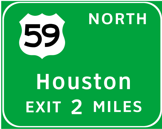
Figure 3-1. Advance Guide sign.
