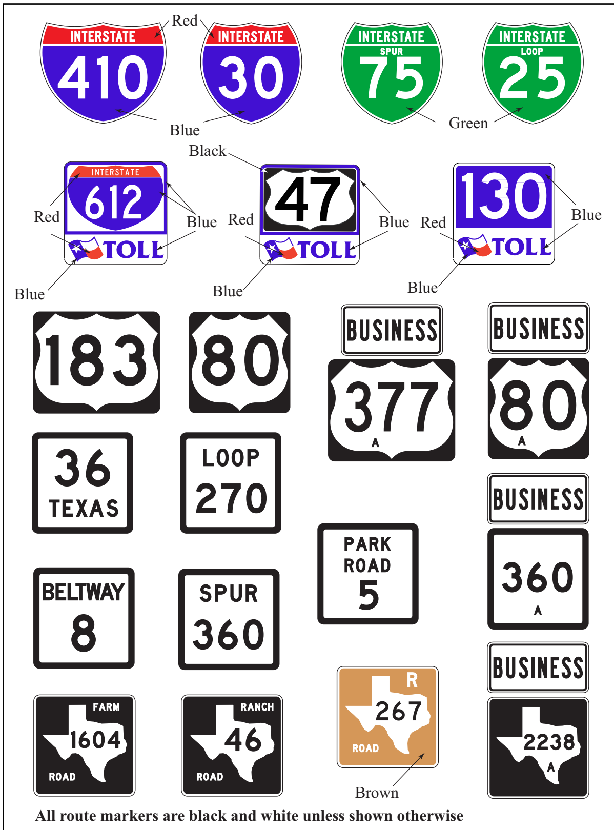
Figure 4-2. Independent ground-mounted Route signs. All route markers are black and white, unless shown otherwise.
