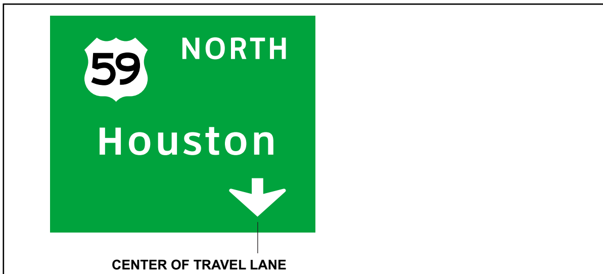
Figure 4-45. Downward arrow placement when sign is not located in the center of the travel lane.
