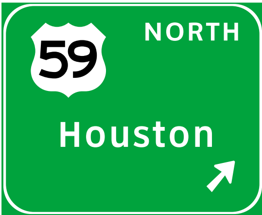
Figure 3-2. Exit Direction sign.
