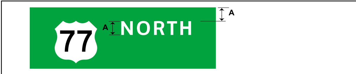
Figure 4-46. Spacing from top border to the nearest line of copy.
