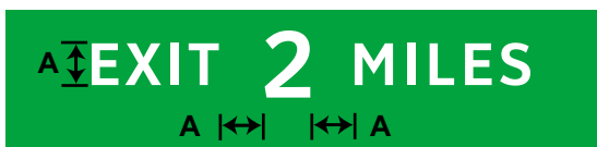
Figure 4-15. Lateral spacing between a word and a mileage numeral.
