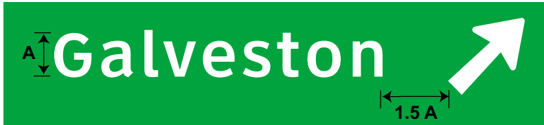
Figure 4-13. Lateral spacing between a word and an arrow.
