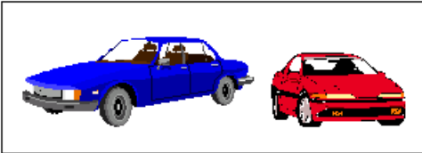
Figure 1-15: FHWA Class 2 — Passenger Cars (With 1- or 2-Axle Trailers)
