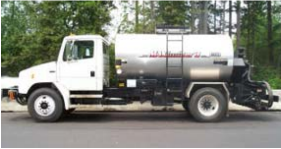
Figure 6-5. Tack Coat Distributor Truck. © Copyright 2006 University of Washington
