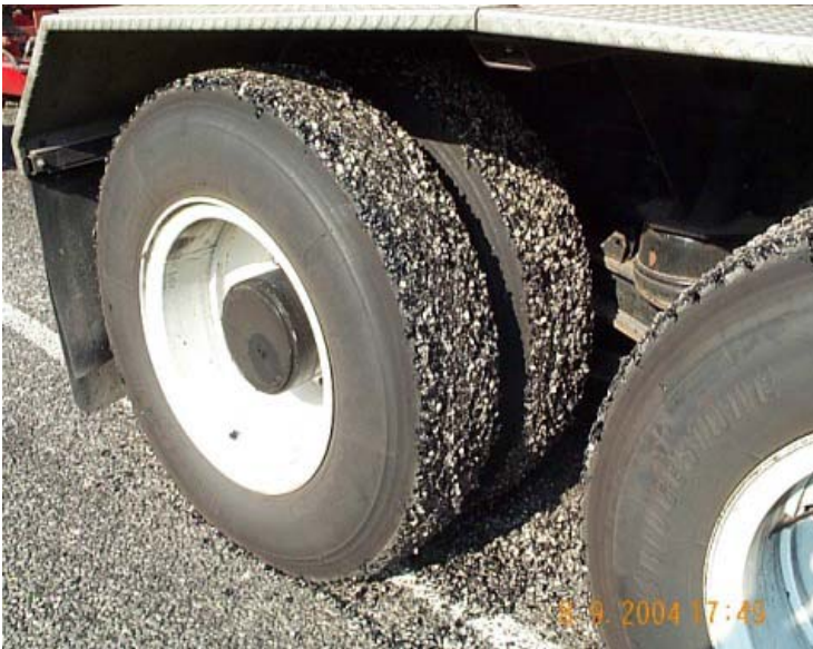
Figure 13-6. Peeling of fresh seal coats (1st photo).
