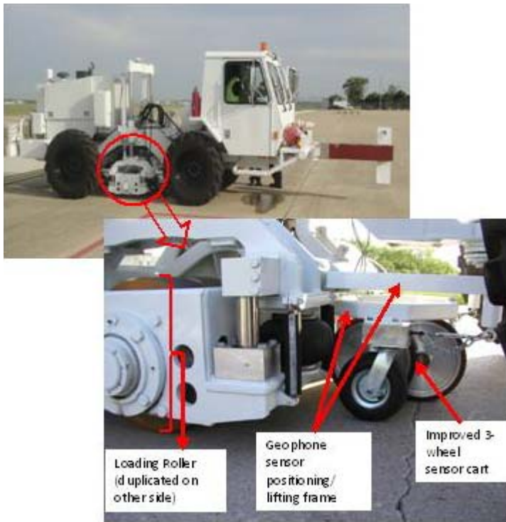
Figure 4-15. Total Pavement Acceptance Device (TPAD) with detail of loading rollers and front geophone cart.
