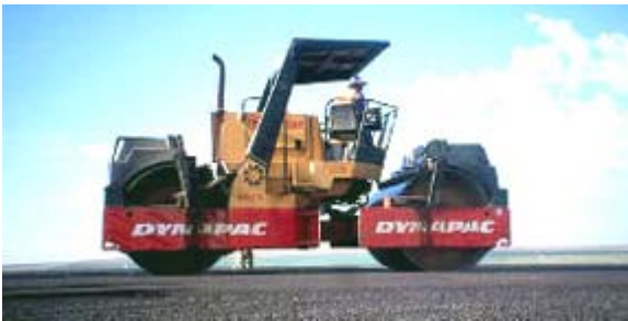
Figure 6-57. Large Vibratory Steel Wheel Roller (18.7 tons 84-inchwide drum). © Copyright 2006 University of Washington
