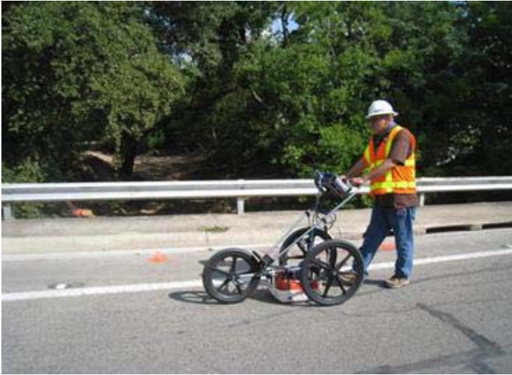
Figure 4-11. 400 MHz Ground-coupled Penetrating Radar.
