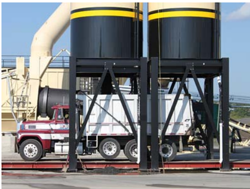
Figure 6-17. Truck loading under a storage silo. © Copyright 2006 University of Washington
