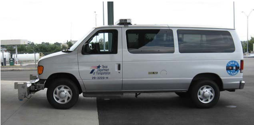
Figure 11-2. High-speed Inertial Profiler with Rut Bar Setup.
