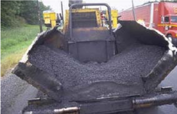
Figure 6-25. Hopper with wings folded up. © Copyright 2006 University of Washington
