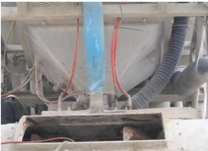
Figure 9-5. Water and admixture supply system.
