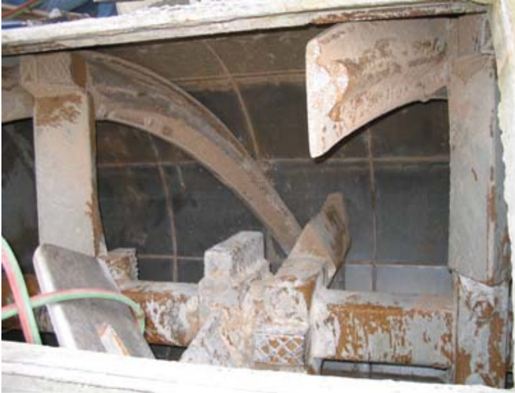
Figure 9-6. Paddles are shown inside a central mix drum.
