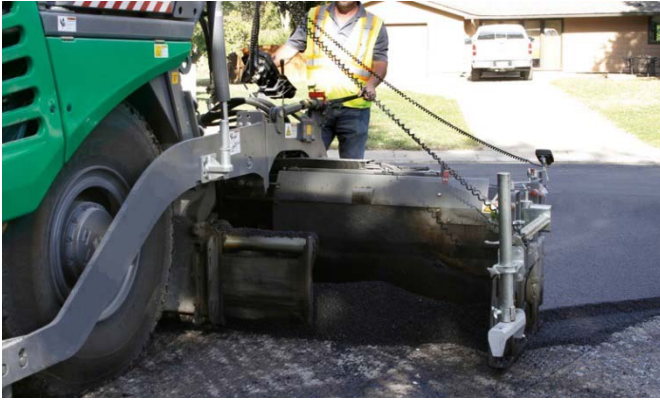
Figure 6-36. Hydraulic Screed Extension. © Copyright 2006 University of Washington
