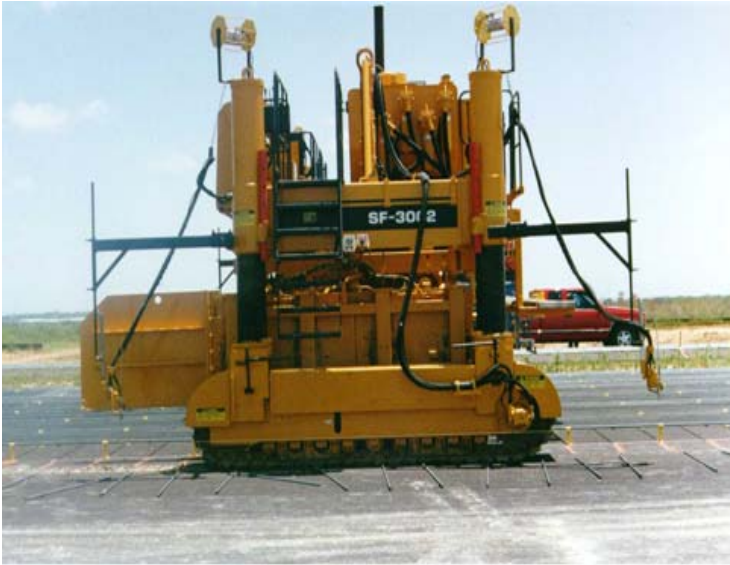
Figure 9-38. Side view of an idle paver.
