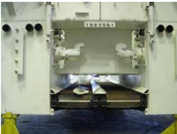
Figure 6-28. Conveyors (seen from the rear of a partially built paver). © Copyright 2006 University of Washington
