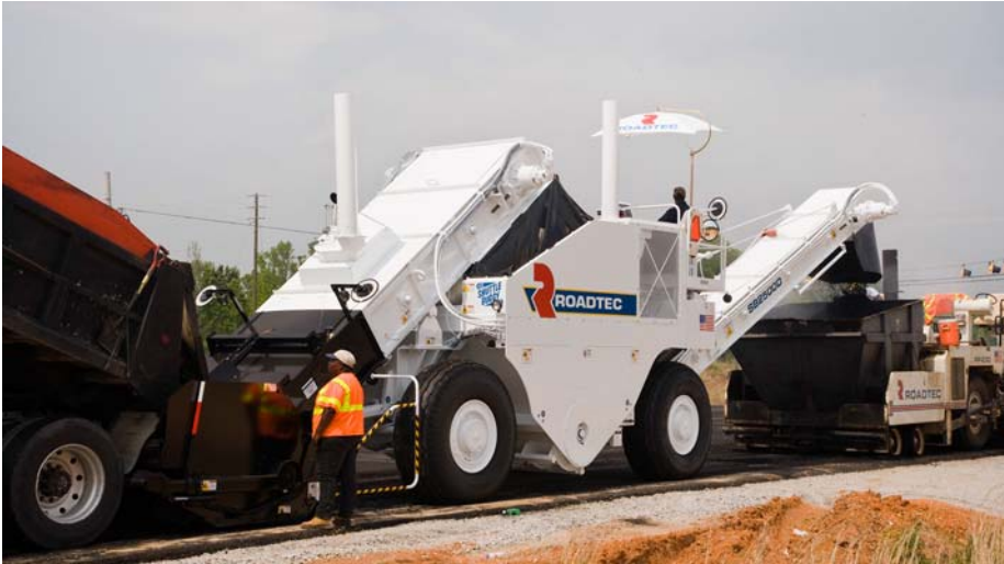
Figure 6-22. Material Transfer Vehicle with surge capacity (Courtesy Roadtec).
