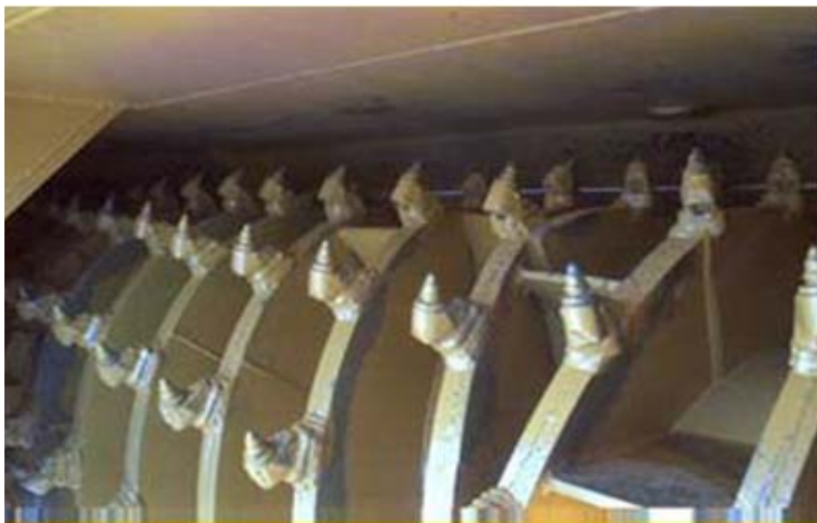
Figure 10-14. Teeth of the Rotomill.
