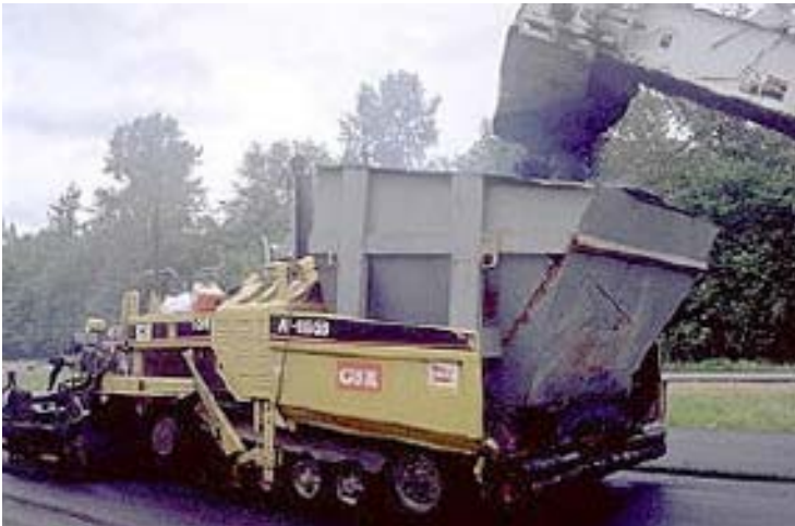
Figure 6-26. Caterpillar AP-1055B with hopper insert. © Copyright 2006 University of Washington
