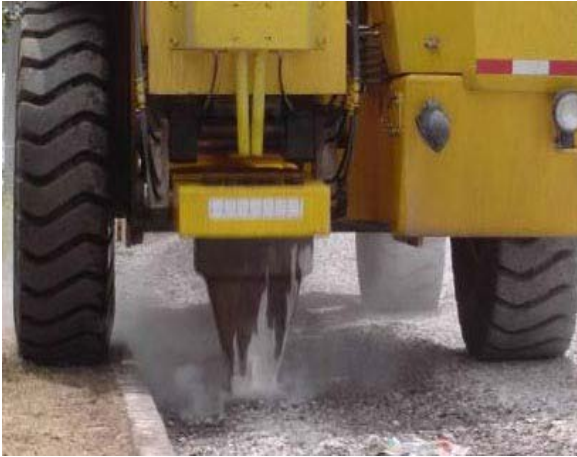
Figure 7-6. Resonant Pavement Breaker. © Copyright 2006 University of Washington
