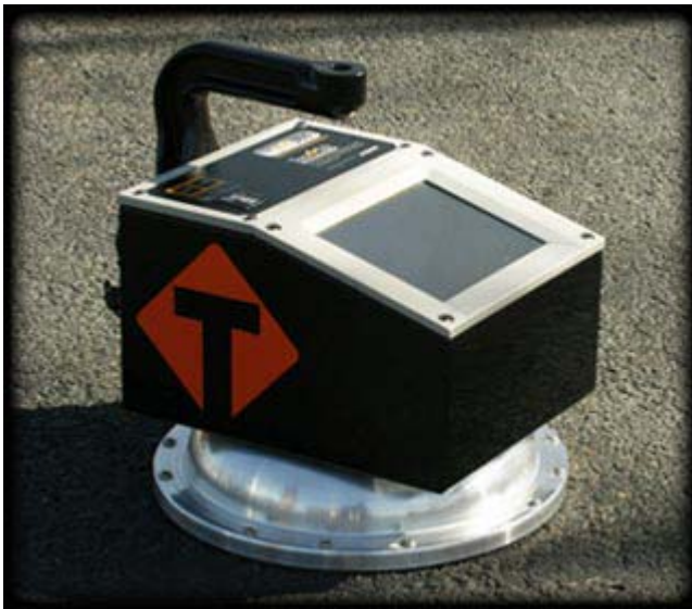
Figure 6-55. Electrical Density Gauge (Courtesy Transtec).
