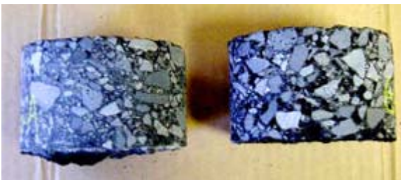
Figure 6-53. Two cores – the core on the right has significantly higher air voids. © Copyright 2006 University of Washington
