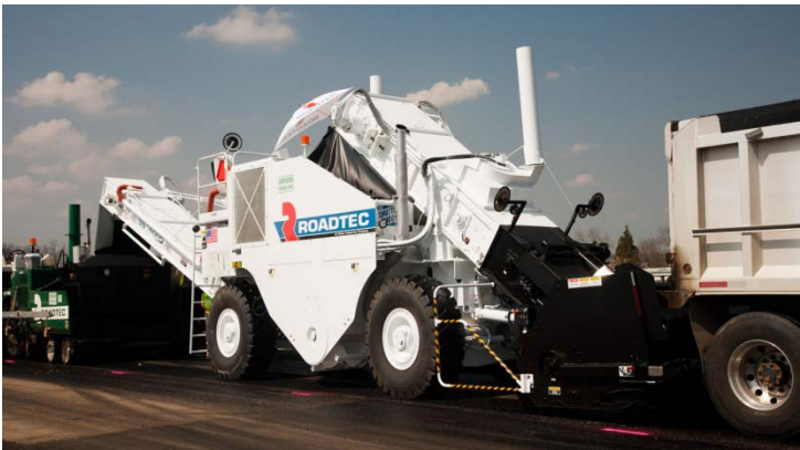
Figure 6-50. Roadtec Shuttle Buggy, front view, showing loading hopper for end dump and live bottom trucks. © Copyright 2006 University of Washington
