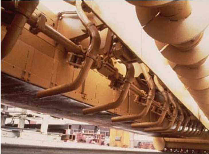
Figure 9-45. Underside of slip-form paver.
