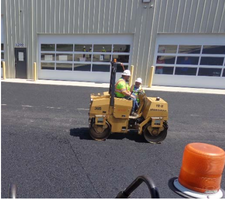
Figure 6-56. Small Static Steel Wheel Roller (1.45 tons 34-inch wide drum). © Copyright 2006 University of Washington
