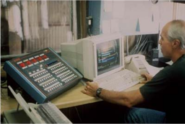
Figure 9-2. Most batch plants are computerized.
