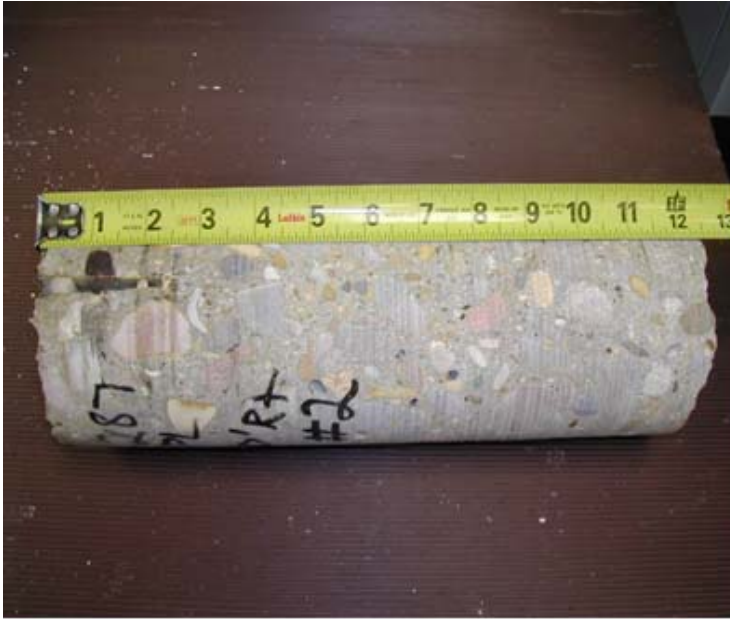
Figure 9-74. Crack was not induced due to shallower saw-cut depth than required.
