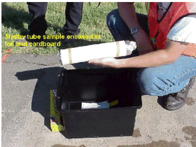
Figure 4-25. Aluminum foil/cardboard tube to protect Shelby tube samples.
